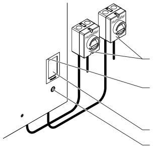
External electrical isolators for heating and control voltage supply (not included in the delivery, must be installed in the mains supply lines)
