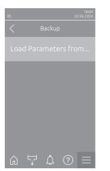
Load Parameters from USB: With this function you can read in parameter settings that were previously saved on a FAT32 formatted USB stick. To do this, the USB stick with the parameter settings must be inserted into the USB interface on the control board. After pressing the selection field, a confirmation dialog appears in which you have to confirm the loading of the parameter settings again.
