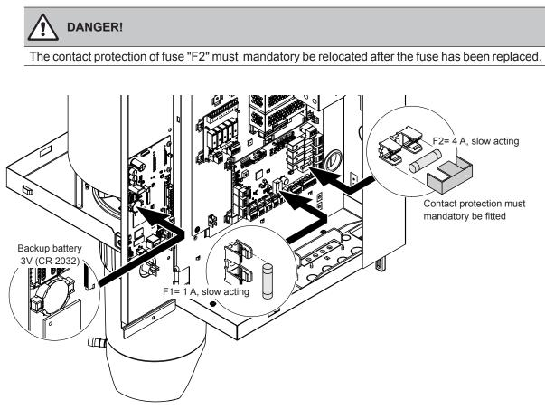
Fig. 6: Position of the backup battery and the fuses on the driver board
