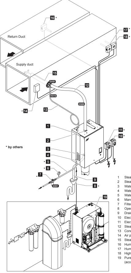
Fig. 2: System overview Condair RS for duct humidification
