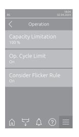
Capacity Limitation: With this setting you determine the capacity limitation in relation to maximum capacity in %.
