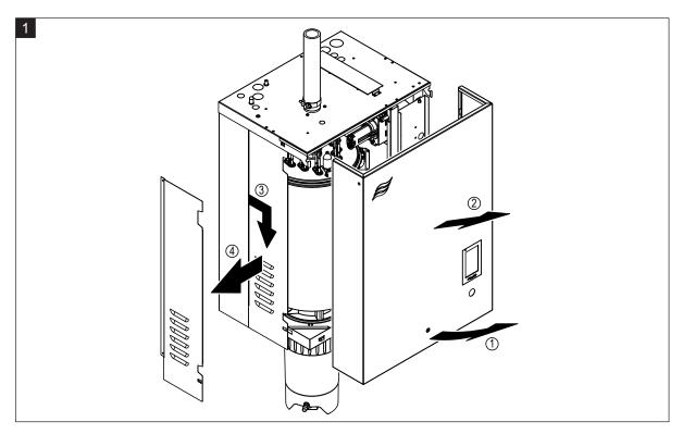
1. Loosen retaining screw on front door or on left front door (for large units) of the unit using a screwdriver, then remove the front door. Pull left side panel to the front and then downwards and remove side panel.
