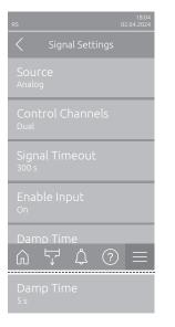
Source: With this setting you determine whether the control signal comes from an analog source "Analog" (humidity sensor, demand signal from an external humidity controller), a BMS (building management system) via "Modbus", "BACnet" or via "IoT".
