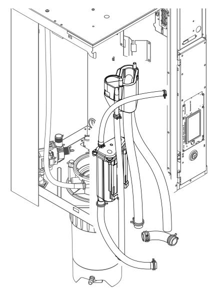
1. Release hose clamps, then disconnect all hoses from the corresponding connectors and remove the hoses.
