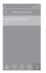
BACnet Protocol: With this setting you can activate ("BACnet MS/TP" or "BACnet/IP") or deactivate ("Off") the communication via the integrated BACnet interfaces.
