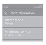
Water Mode: With this setting you determine whether the flushing interval time and the maintenance interval time for the small and the extended maintenance are calculated automatically on the basis of parameters water quality and water hardness (Setting: "Calculated") or whether the flushing interval time and the maintenance interval time for the small and the extended maintenance can be set manually (Setting: "Manual").
