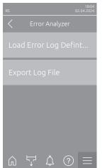
Load Error Log Definition (carried out ex works): With this function you can load an "Error Log Definition file" available from Condair on a USB stick for recording malfunctions. Once the "Error Log Definition file" has been loaded, an error log file is created as soon as an error occurs during operation. This file can then be saved on a USB stick using the "Export Log File" function.
