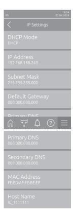
DHCP Mode: With this setting you determine whether you want to assign the IP Address, the Subnet Mask, the Default Gateway as well as the Primary and Secondary DNS address as fixed values or whether these should be dynamically assigned via a DHCP server.
