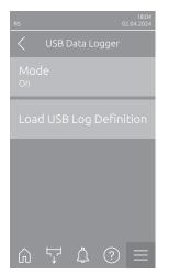
Mode: With this function you can switch the operating data recording on a USB stick on or off. A new csv file is created for each day and stored on the USB stick.
