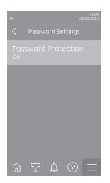
Password Protection: With this function you can protect the access to the main menu with the user password "8808" against unauthorized access ("On") or not ("Off").
