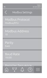
Modbus Protocol: With this setting you can activate "Modbus/RTU" or "Modbus/TCP" communication via a Modbus network or deactivate ("Off") Modbus communication.
