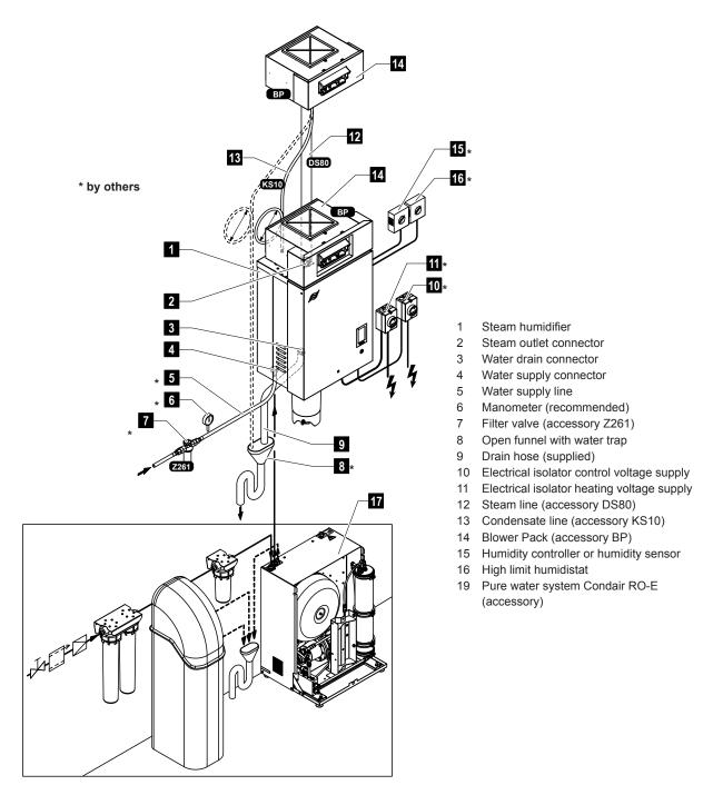
Fig. 3: System overview Condair RS for direct room humidification
